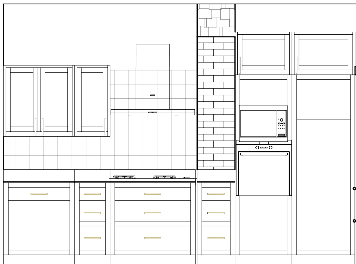
2 Interior Elevation - Kitchen Scale: 1/2" = 1'-0"
