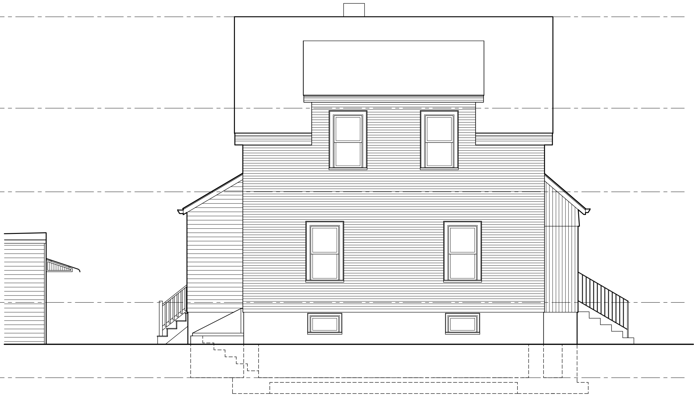
2 EXISTING EAST (SIDE) ELEVATION 3/16"=1'-0"
