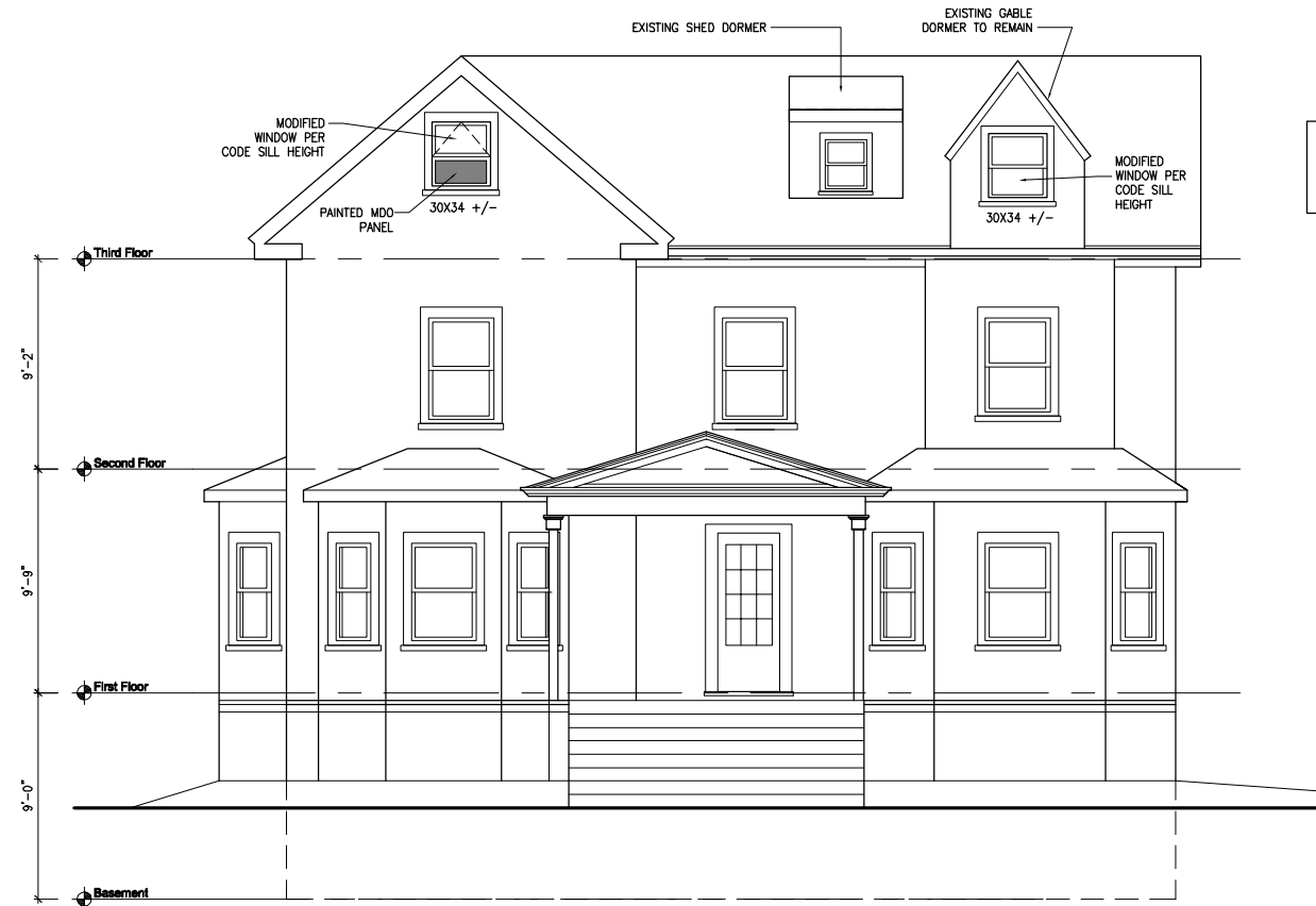
1 FRONT ELEVATION - NORTH Scale: 1/4" = 1'-0"
