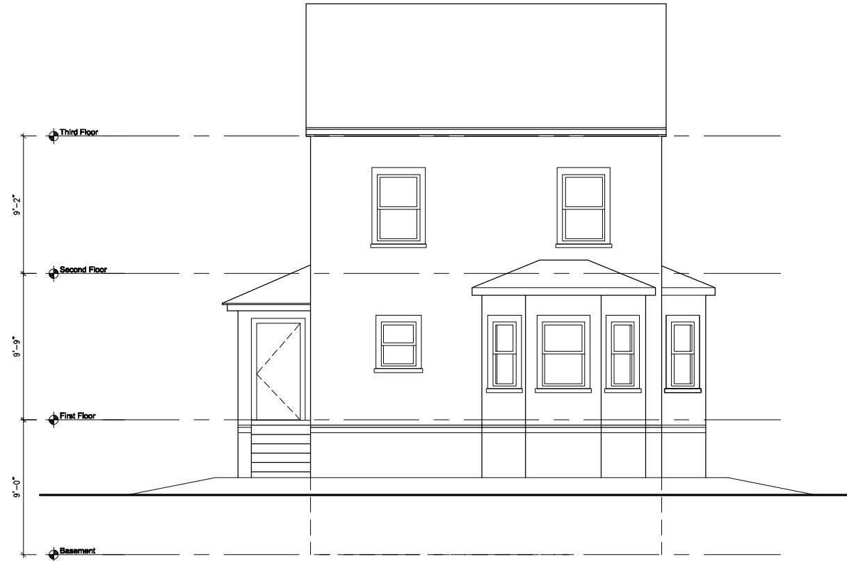
2 SIDE ELEVATION - EAST Scale: 1/4" = 1'-0"
