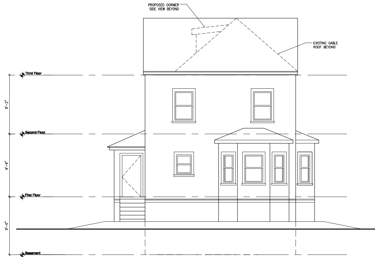
2 SIDE ELEVATION - EAST - NO CHANGE Scale: 1/4" = 1'-0"
