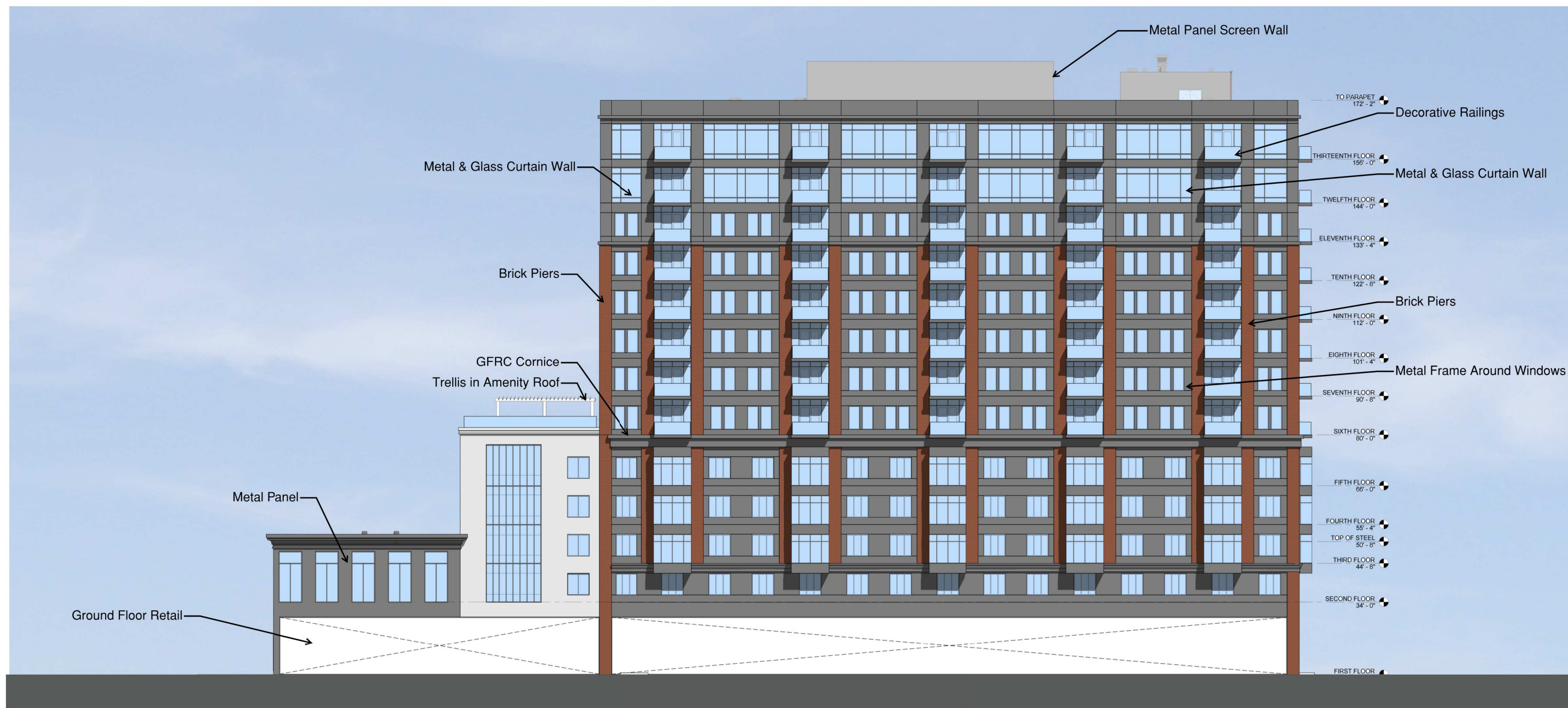
East Elevation: Assembly Row
