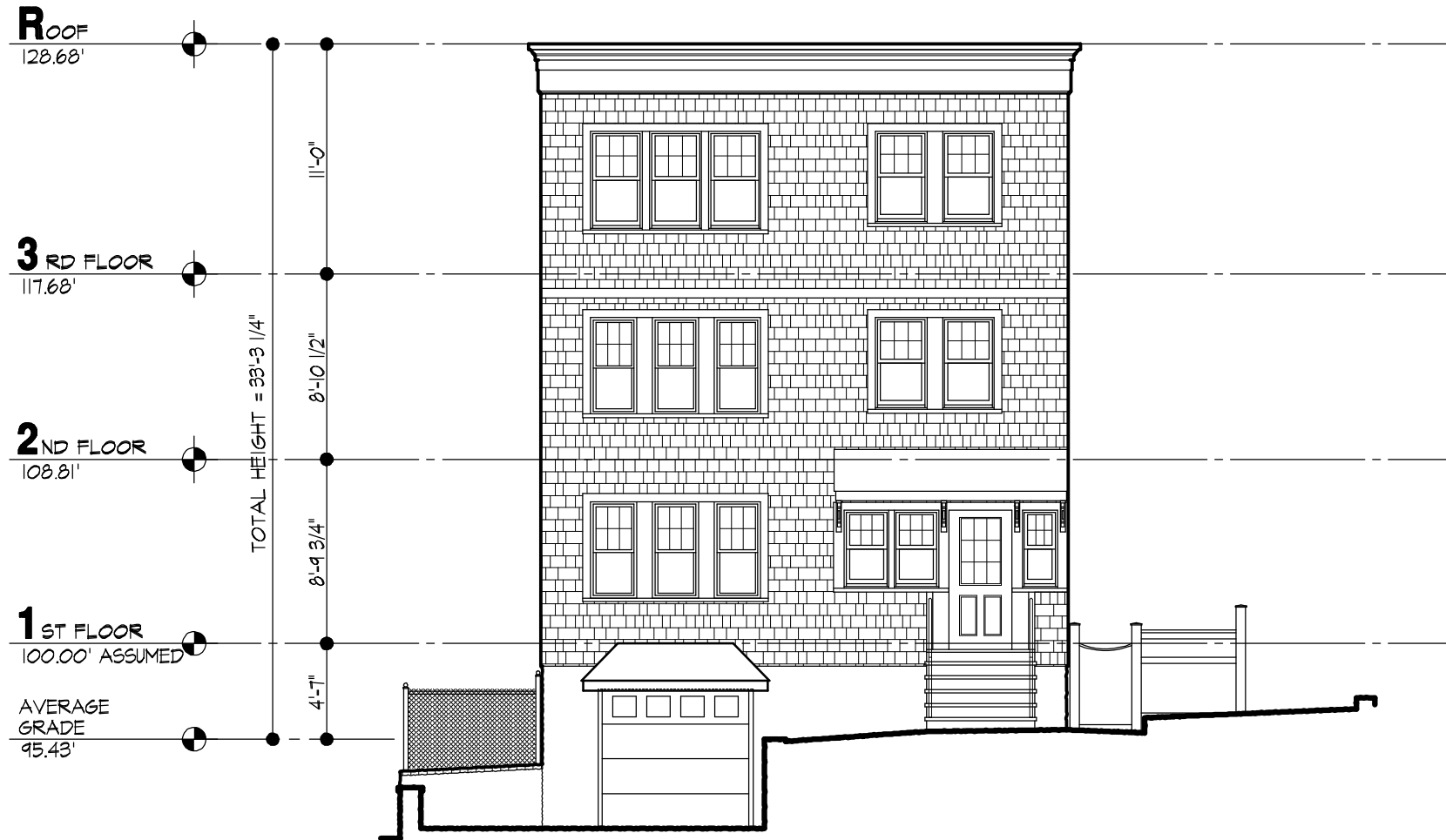
1 A2.1 FRONT ELEVATION 1/8" = 1'-0"
