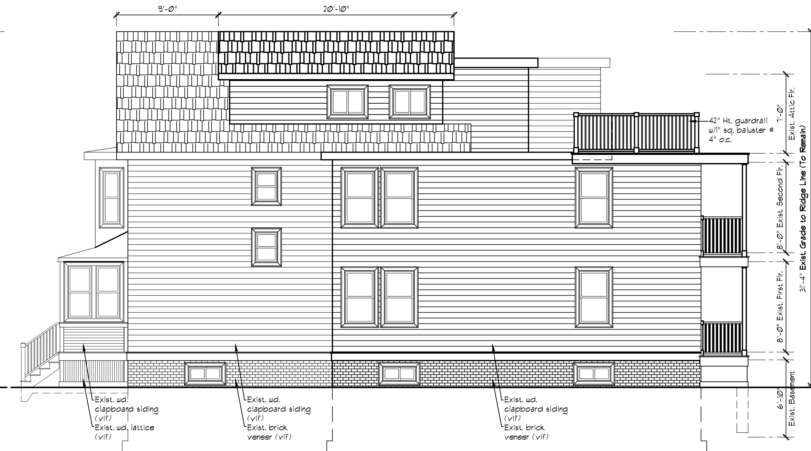
2 A-1.1 Proposed Exterior Elevation (Right) SCALE: 3/16" = 1'-0"
