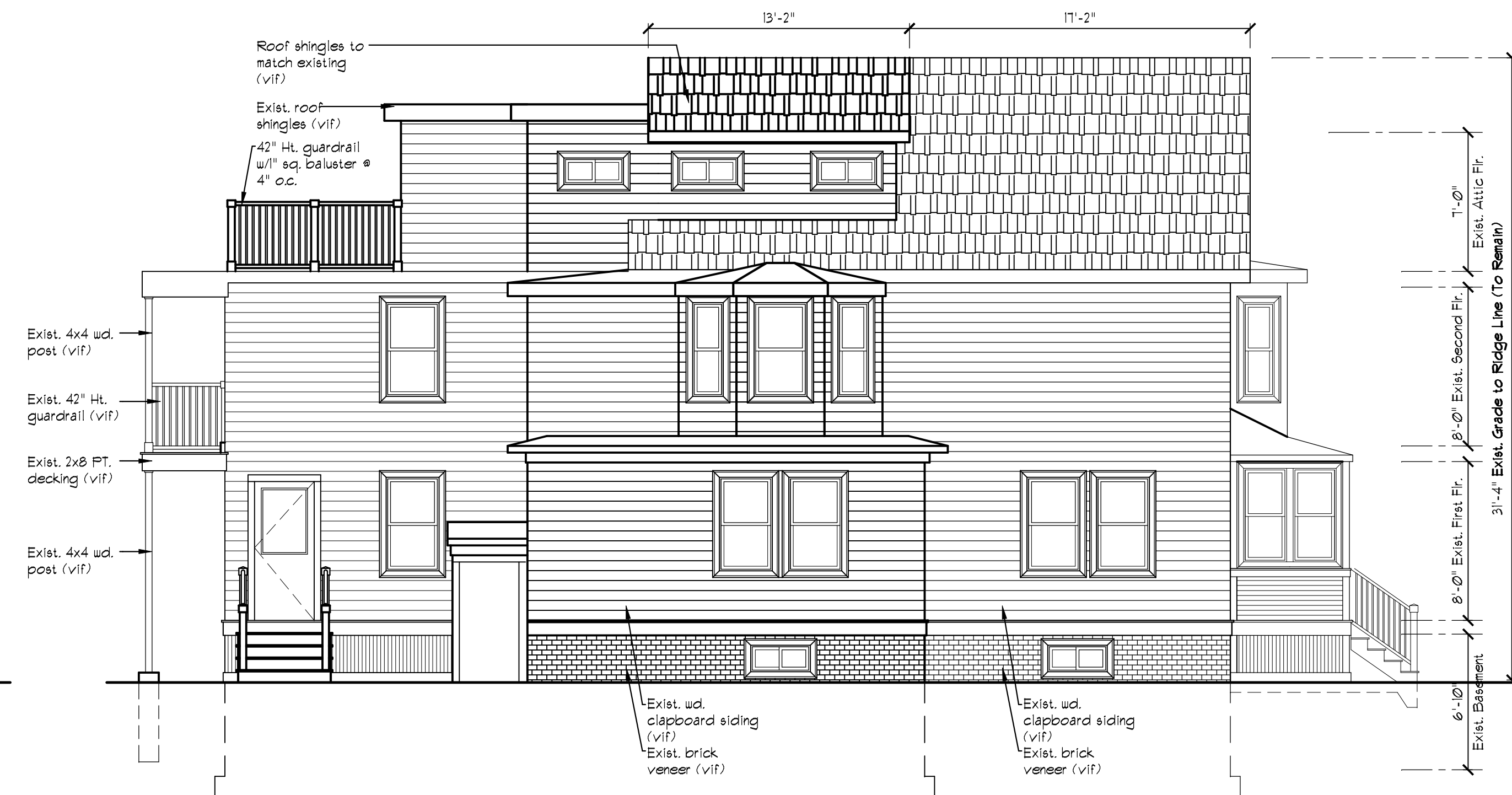
3 A-1.1 Proposed Exterior Elevation (Left) SCALE: 3/16" = 1'-0"
