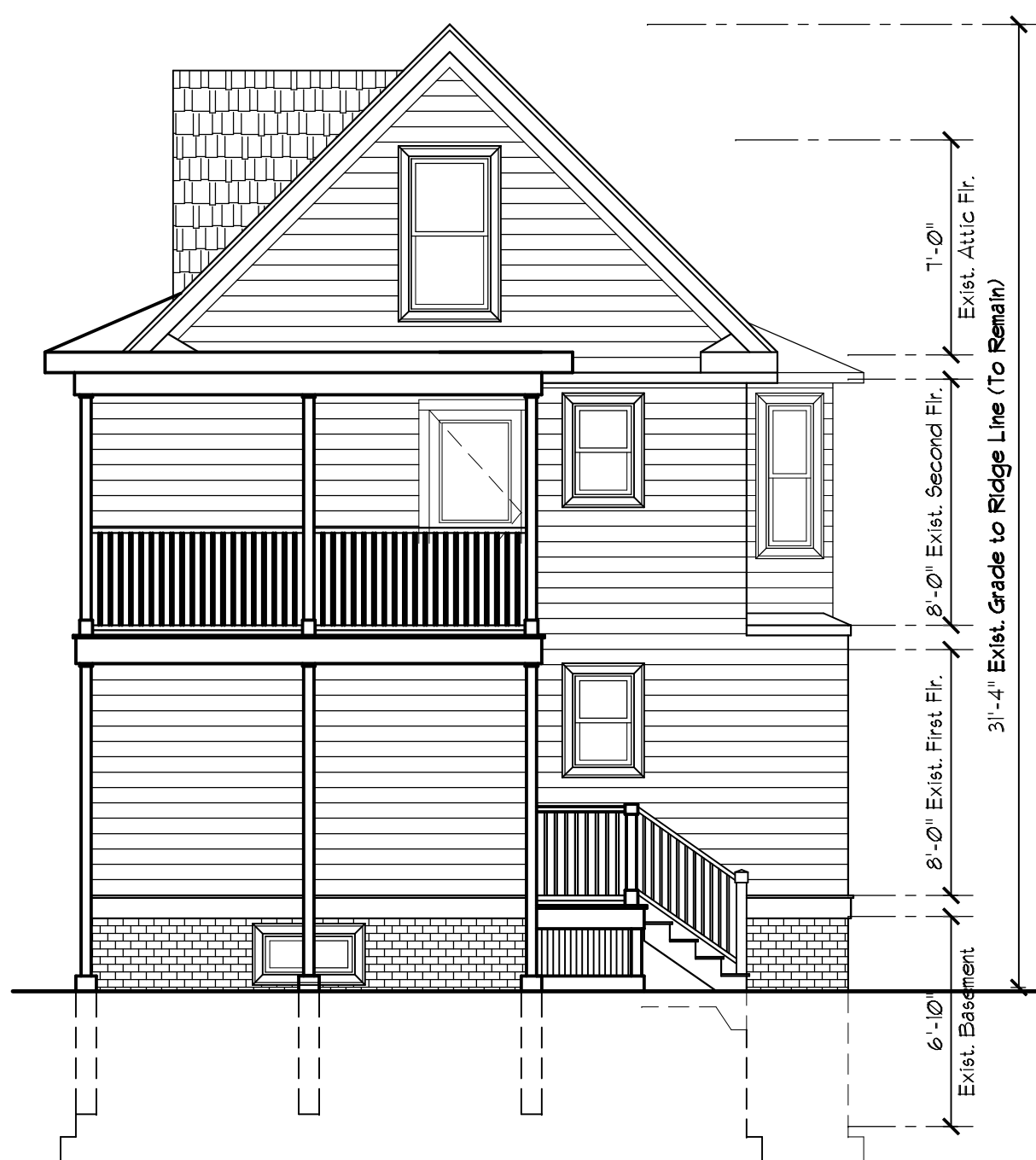
4 Existing Condition Exterior Elevation (Rear) EX-1.1 SCALE: 3/16" = 1'-0"
