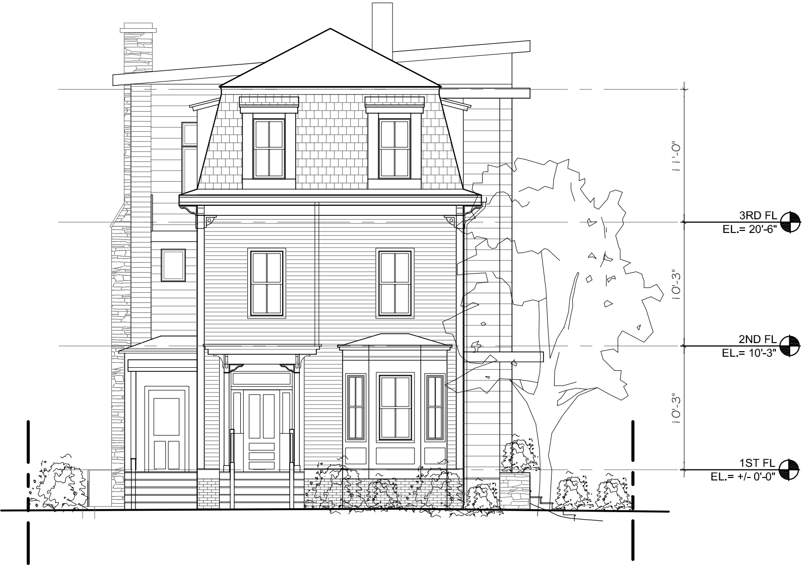
1 FRONT ELEVATION SCALE 1/8" = 1'-0"
