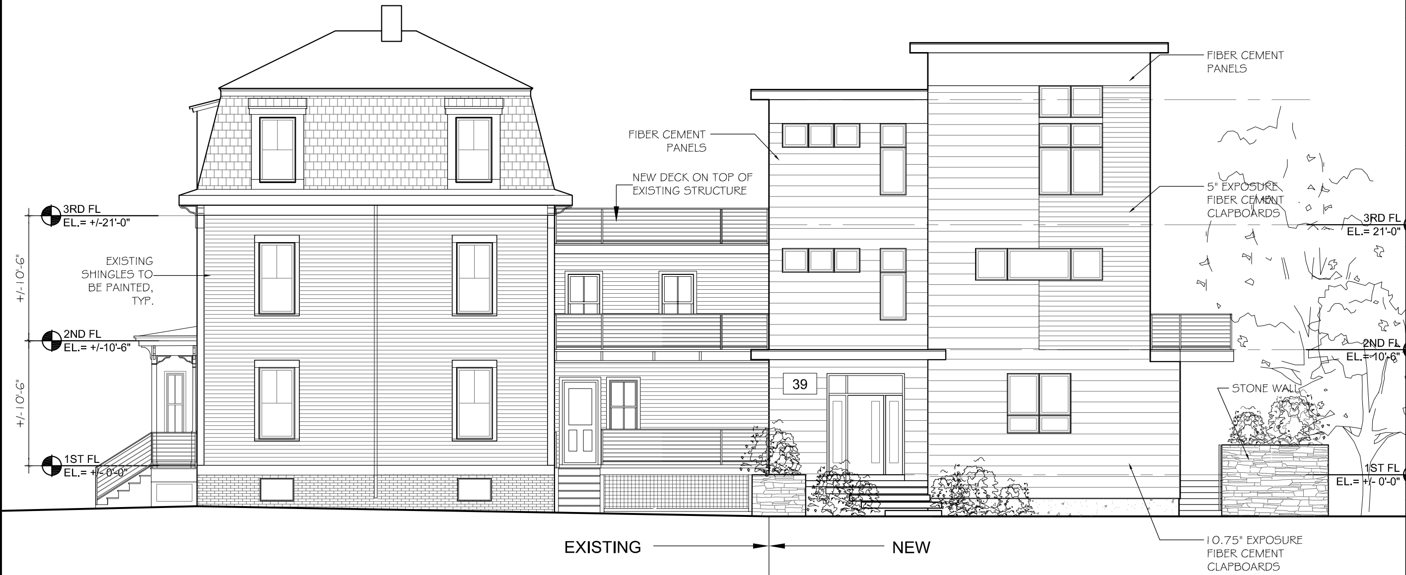
1 RIGHT ELEVATION SCALE 1/8" = 1'-0"
