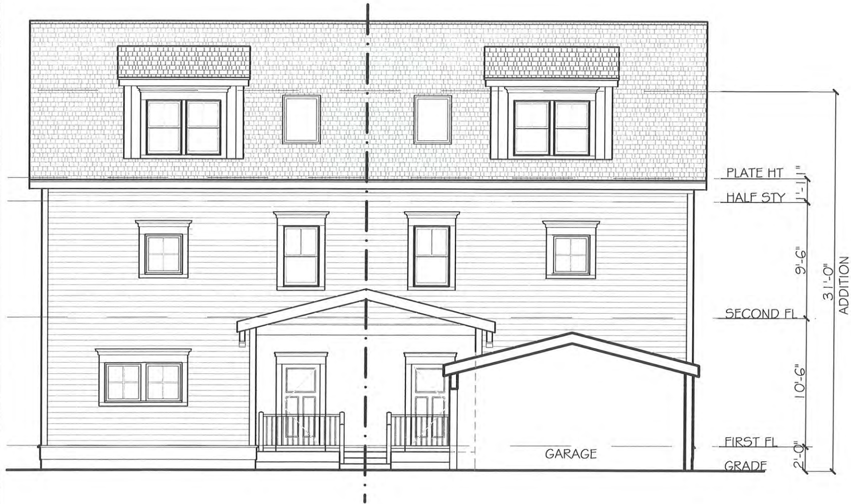
1 FRONT ELEVATION (ADDITION) SCALE: 1/8"=1'-0"
