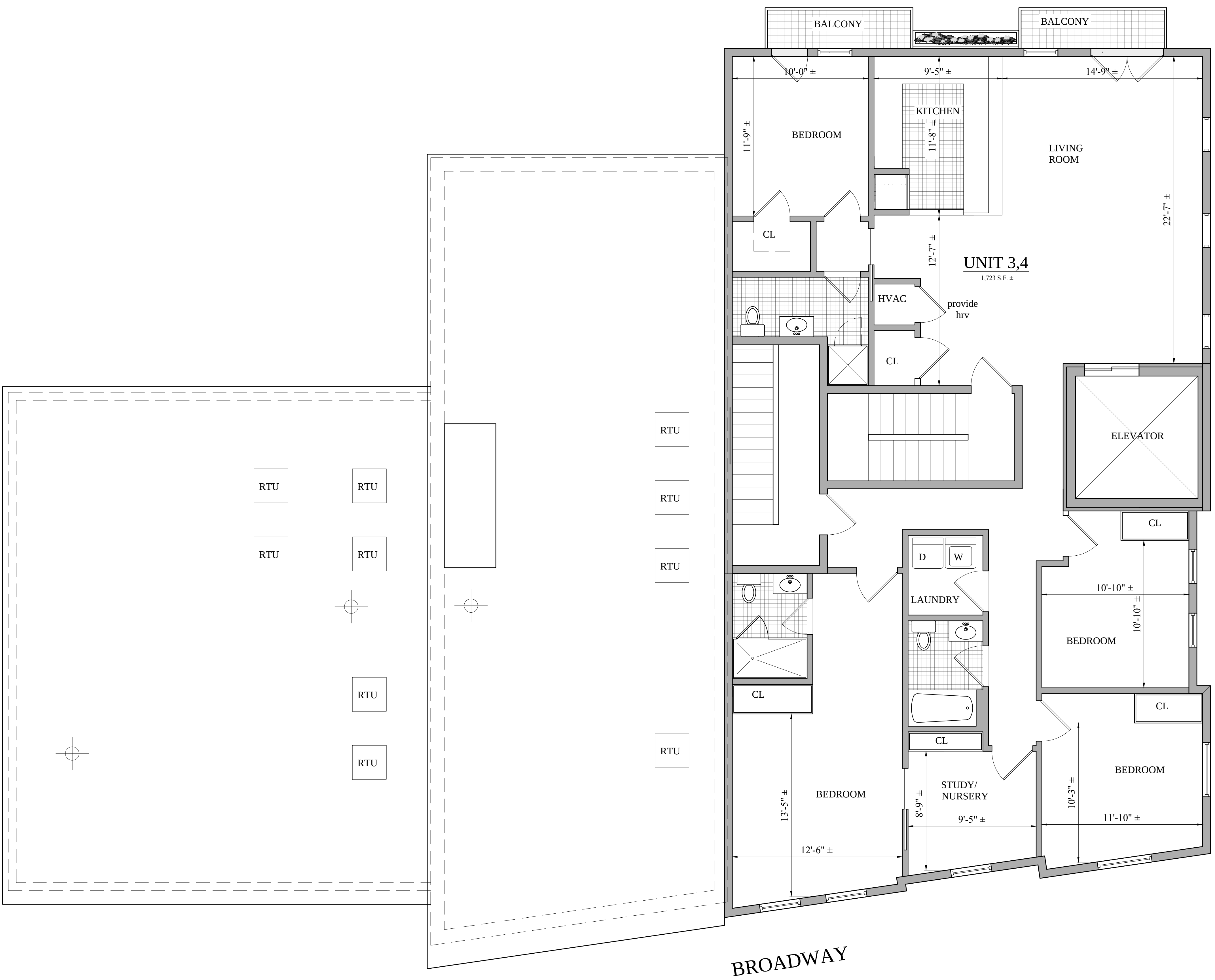
5 PROPOSED 4TH FLOOR PLAN 1/4" = 1'-0"
