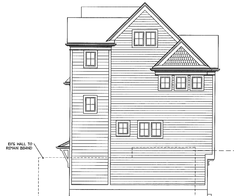
PROPOSED BLDG 3 NORTH ELEVATION
