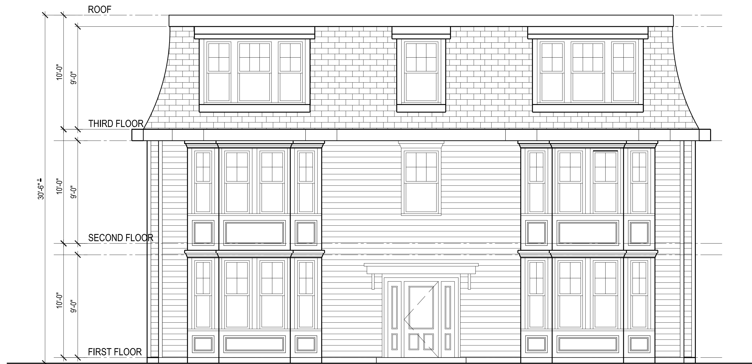
1 NORTH ELEVATION A-300 Scale: 1/4"=1'-0"
