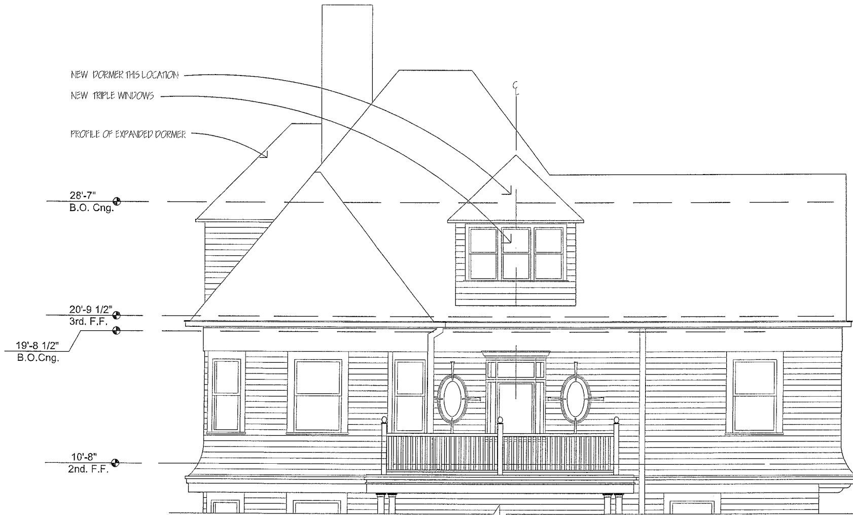
1 Partial East Elevation A-2.02
