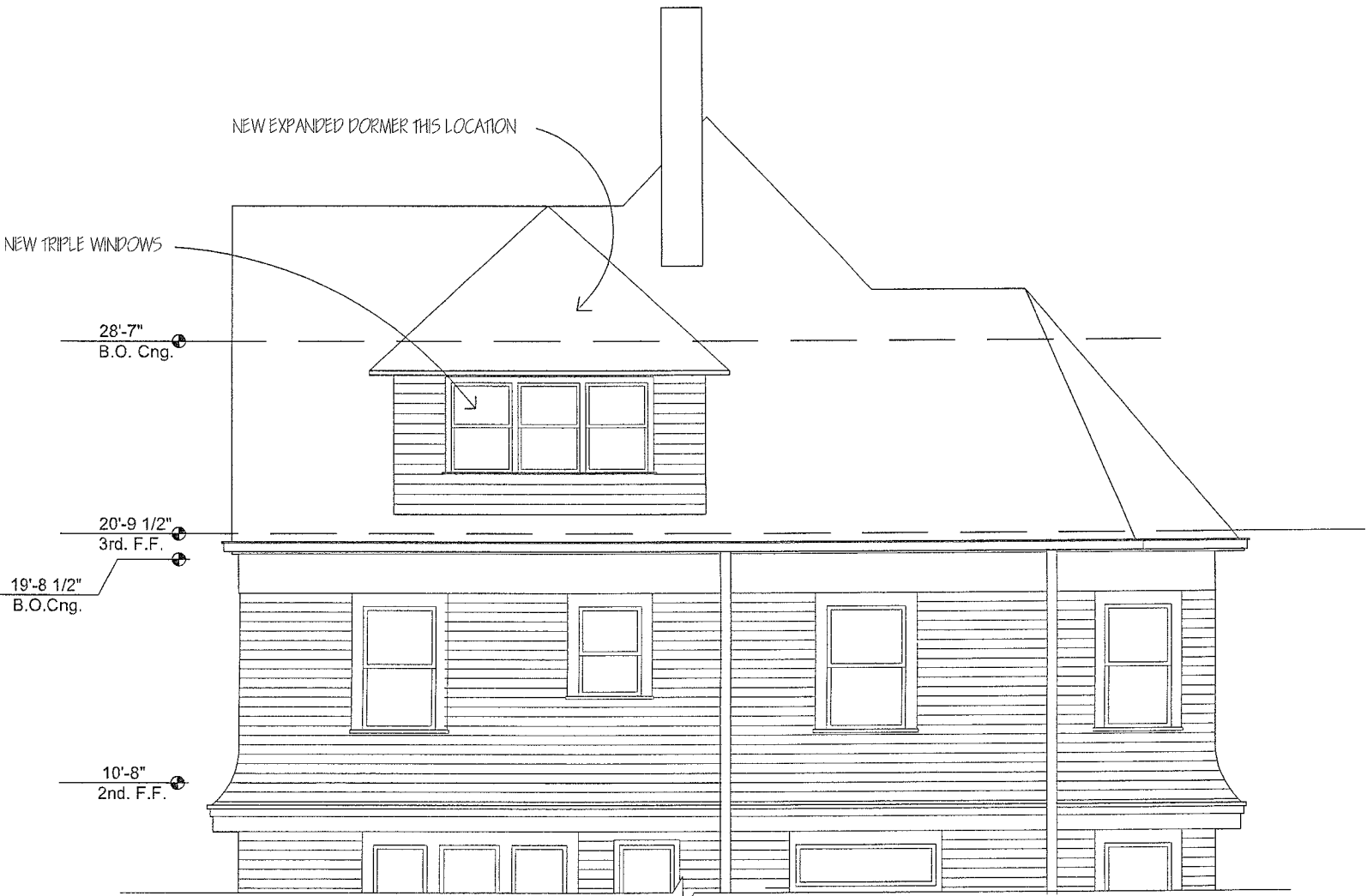
1 Partial South Elevation A-2.01
