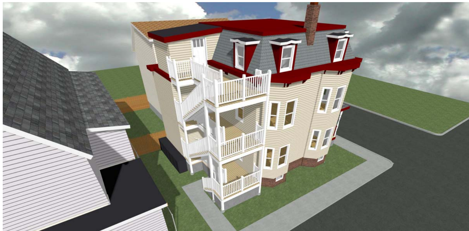
Aerial View of Proposed Decks and Stairs
