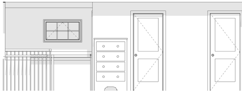
⑦ BEDROOM ELEVATION AT BATH & STAIR 1/2" = 1'-0"
