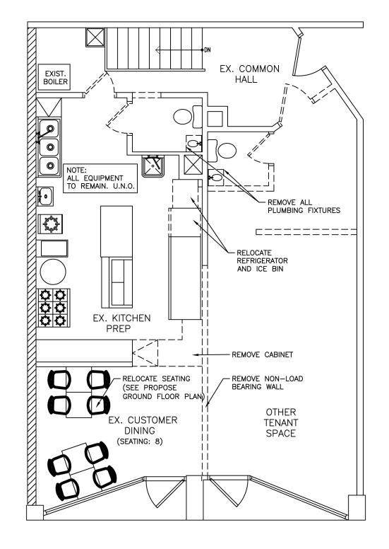
EXISTING/DEMOLITION PLAN scale: 3/16" = 1'-0"
