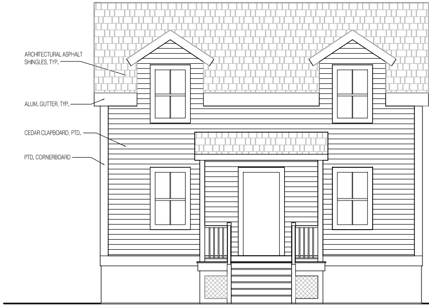
6 WEST ELEVATION - BUILDING "B" SCALE: 1/8" = 1'-0"
