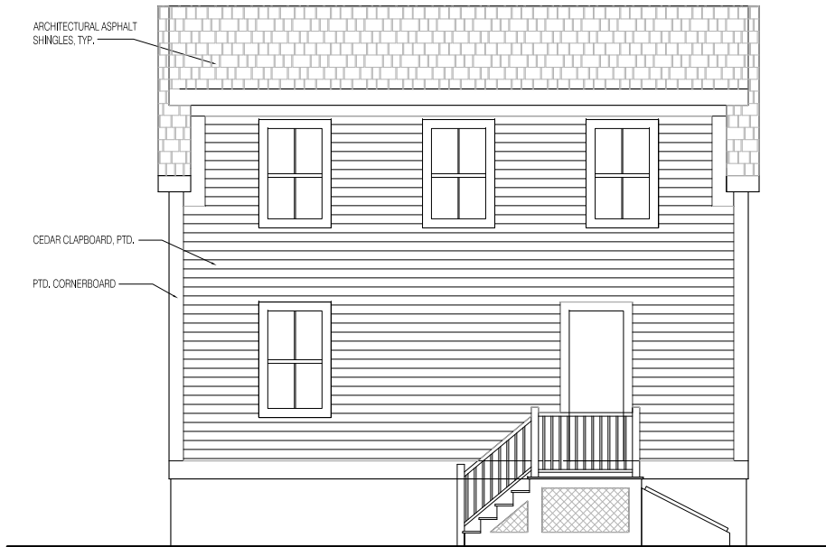
3 EAST ELEVATION - BUILDING "B" SCALE: 1/8" = 1'-0"
