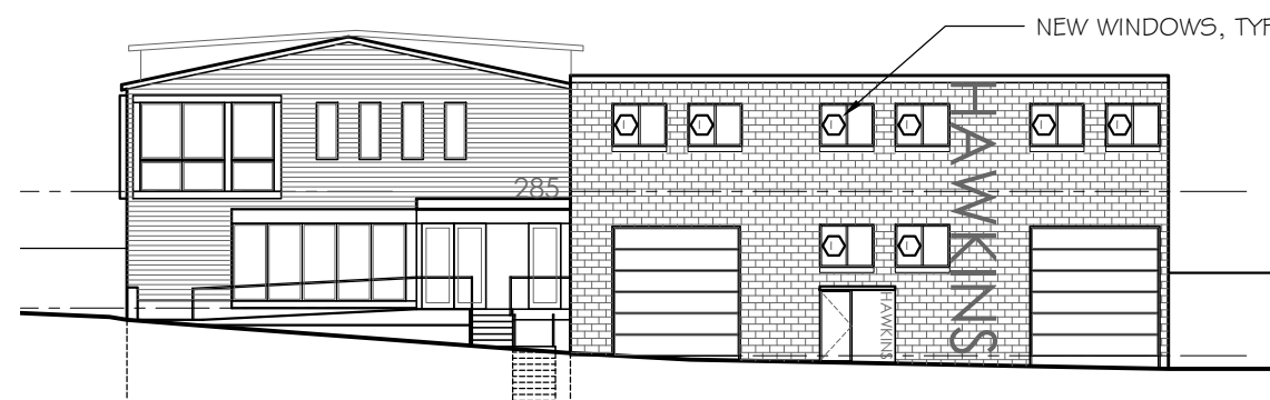
3 SIDE ELEVATION (PHASE 2) SCALE 1/20" = 1'-0" HAWKINS ST
