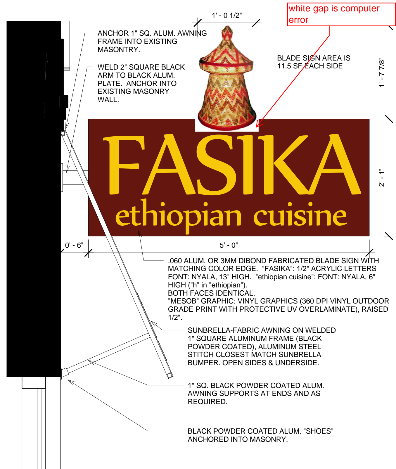
2 Awning Section and Blade Sign Elevation 1" = 1'-0"
