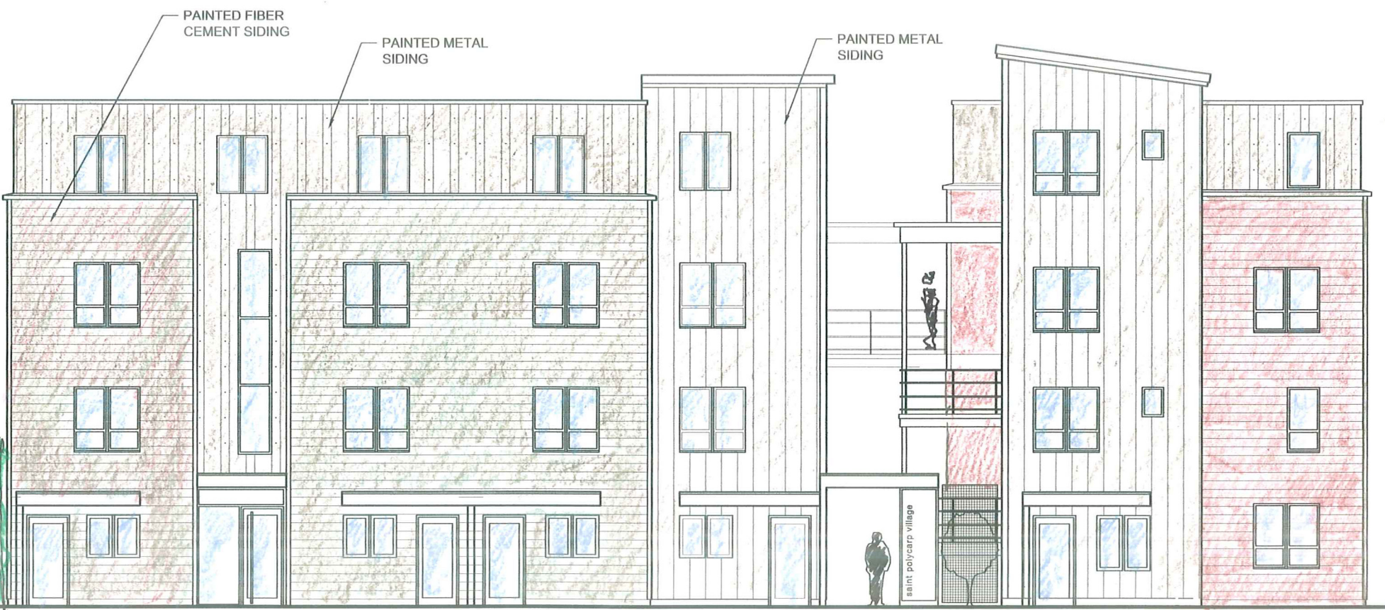
ELEVATION 6 BUILDING F
