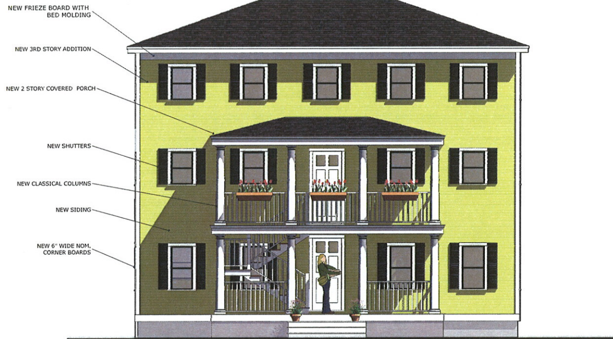
1 REVISED SOUTH ELEVATION 1/4" = 1'-0"
